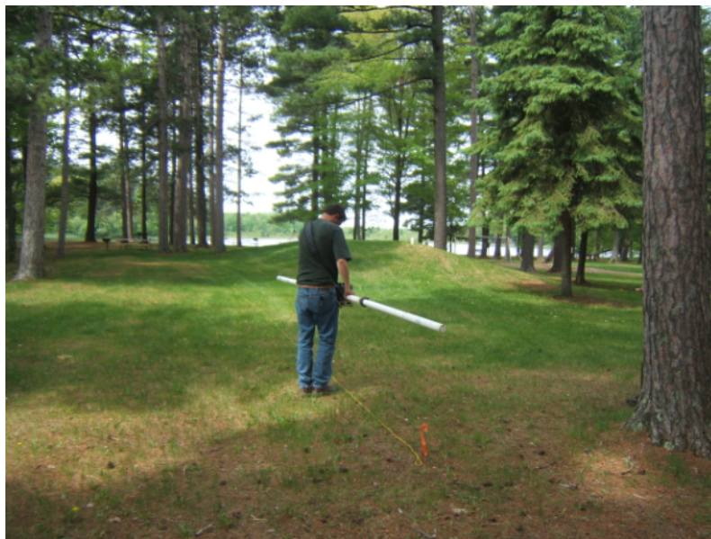
Figure 3: Use of a Geonics EM31 conductivity meter to investigate the effluent plume beneath a Wisconsin mound at Lake Collins Campground, Wisconsin.
